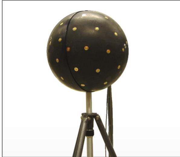
**Figure 6.1:** The test model of the Spherical Harmonics Beamformer, having 64 microphones.
